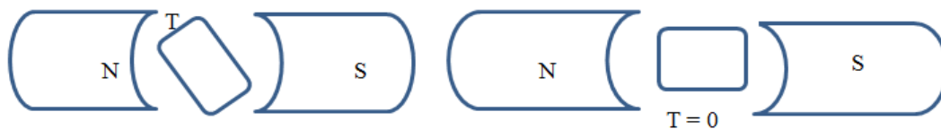
Rotor Position due to Revolving Magnetic Field
